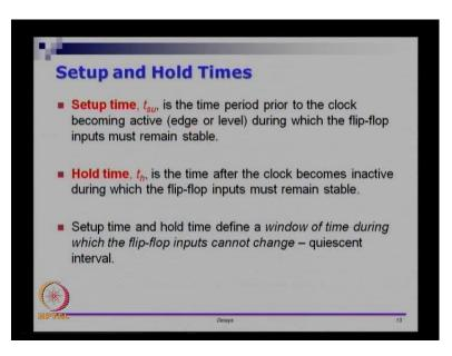
So, let us see what the definitions are. Set up time usually refer to as t subscript su; is the time period prior to the clock. Remember, we are talking about sequential elements here. So, there is always the notion of clock when we talk about sequential elements. So, t s u is the time period before the clock becoming active, during which the inputs to a flip flop
