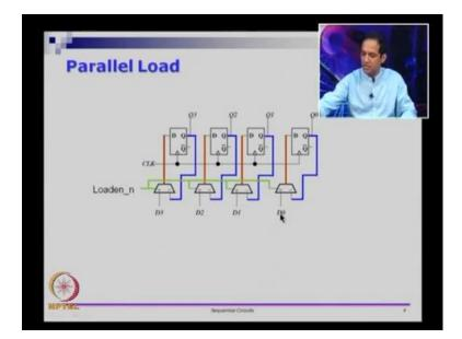
We start with the register that we had earlier. So, we have these four flip-flops, which make the register. So, the D inputs are not shown now. What we are going to provide is you are going to provide a control signal called load enable. This load enable signal – if load enable is 1, we want something to be loaded from the external world; we want to copy something from the external world. If load enable is 0; we want to retain the previous values that we had for Q 3, Q 2, Q 1 and Q naught.
