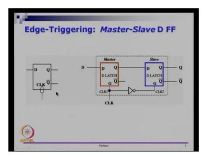
We will see how these circuits come about and so on in one step after the other. The first thing is the symbol for a flip flop is usually drawn as a rectangle like this and D input and there is Q and Q bar. And in a latch, we actually had just a single line coming in and we called it Clk. Now, we also have a small traingle kind of thing here. So, forget the bubble for a while now, we also have a triangle kind of a thing, that is indicating that, it is a flip flop.
