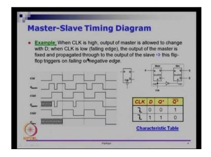
So, let us see a quick timing diagram. What you are seeing is, you are seeing the same circuit here and the symbol for that circuit is here. So, I also put the bubble here, because the bubble is necessary and let us see, how the circuit will work. So, I am assuming that Clk is a periodic signal, so that is coming an on and off at some regular intervals. So, let us assume that this is some time line, this is some time line and so on.
