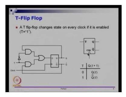
Then, let us look at a circuit called T flip flop, T flip flop is an interesting circuits. So, T flip flop is actually a minor variations of the D flip flop. So, let us look at the circuit, you have a D flip flop and there is some circuitry here, the circuitry is actually doing the function of a mux or a multiplexer. So, if you describe the output of this OR gate in terms of the inputs namely T, Q and Q bar, we can see that this OR gate is doing T bar and Q or T and Q bar.
