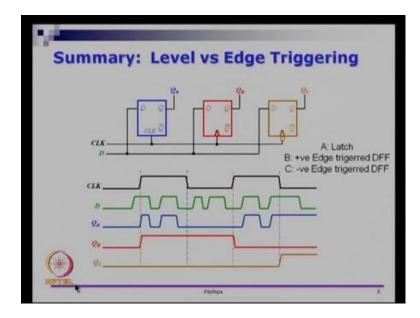
So, in this circuit, I have three difference logic elements sequential elements on the left side, you have a latch. So, latch is just D, Q and Q bar and an enables signal that comes in. And in the middle is the red one which is actually a positive edge trigger D flip flop. So, this flip flop will capture D, whenever the clock signal goes from 0 to 1, otherwise it will ignore the changes in D, it keep the values of Q and this brown one is the negative edge trigger D flip flop.
