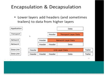
And this actually explains how the communication theory happened so the data the transport layer attaches the better and it converts the data into a transport layer data and then when it goes to the network layer Network layer adds more headers it takes the whole thing the network layer data and then if you look at it actually, it is it has this the transport layer header and then the pita and then the data link layer.
