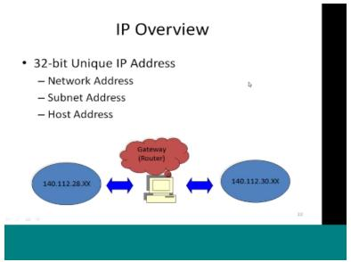
So now we will be going into the IP overview. I just wanted to give some basic overview of the IP addresses so here there are three different things basically make them network address subnet address and the host address then basically read up the numbers that normally encounter like one party dot told 112 dot 28 dot something and then how would that connects to the other ones and then we the Gateway.
