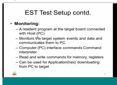
So what is monitoring? Monitoring as an output activity from the target system used for embedded system testing so what are the elements used to be monitoring is the resident program that is based system which is connected with the hoist as I said the connection could be RS232 or it could be any of the interface system. The interface could be generally used or can is used in many places control area.
