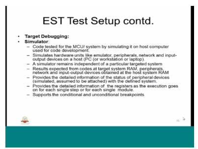
So, target, the embedded system target can be tested with the help of simulator so in simulation what it has basically, it uses the knowledge of target processor or make it controller or target system architecture at the host side that means on the host processor.
