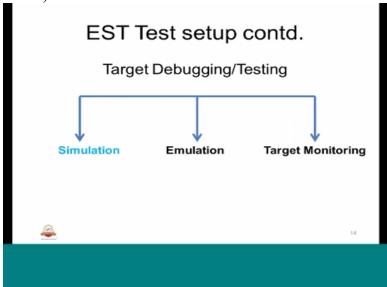
Those are broadly three categories having said that we use different setups for the development and testing. The setup is broadly categorized in three ways testing in which simulation, testing with emulation and with the help of target monitoring that means the target debugging testing is categorized simulation, emulation and target monitoring. What are those? So we will see each one.
