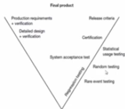
Figure 3.4 Allocation of test related issues on the development cycle of the final product
