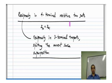
So, this is proved basically we have proved that Z 1 to equal Z 2 1 and in doing that we used reciprocity in three terminal resistive two ports. And we also use the earlier theorem on splitting the current source and super position, because we are using reciprocity in three terminal 2 ports we had to define some other ports with a single common node as the reference node and we were able to do that quite easily hope that is clear.
