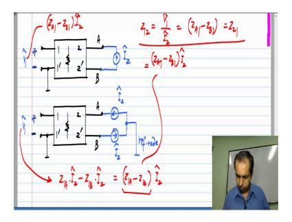
Now, in the original case I have both of these sources being active, so the actual voltage V 1 hat would be the sum of this voltage and that voltage. So, the voltage here would be Z 1 A times I 2 hat minus Z 1 B times I 2 hat or Z 1 A minus Z 1 B times I 2 hat. So, pretty simple I split the current source took 1 current source at a time got the outputs and I have this as my output at port 1 when port 2 is exited.
