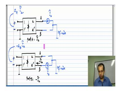
So, now, since I have two sources here I leaves super position, so I will split this into two cases, where I have only the upper current source active over there and only the lower current source active over there. Now, what is the voltage I get at port 1, so now, port A is fed with I 2 hat, so at port 1 I will get Z 1 A times I 2 hat with only this current source being active, if you look at the lower picture port B is exited with minus I 2 hat, because
