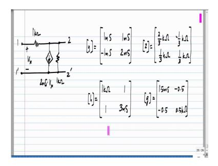
For instance, this is another circuit and in this case certainly y 1 1 is not equal to y 1 2 and z 1 1 is not equal to z 1 2 and so on. So, they have some numbers which are not necessarily equal to each other. So, there does not appear to be a special relationship between the forward and the reverse parameters in this case. Now, ((Refer Time: 02:56)) as part of activities or assignments you would have solved for the two port parameters of other networks, which
