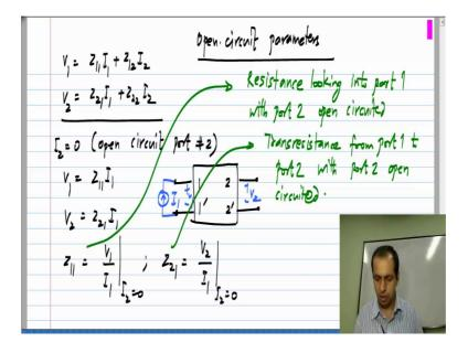
Now, let say you are given a network and you are asked to find the Z parameters, you need four measurements. Because, you have four parameters and by taking four possible combinations of I 1 and I 2, you will get four equations, you take four possible combinations of I 1 and I 2 measure V 1 and V 2 for each case, you will get four equations and that is it, from that you can solve for the four parameters.
