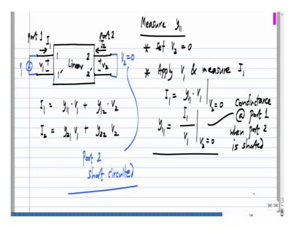
In other words, What is the meaning of setting V 2 to zero we short circuit the second port. So, you short the second port and essentially measure the conductance looking in to the first port, because when you short circuit the second port this whole thing. We just have these two terminals to play with we apply a voltage and find the current going there take the ratio of current voltage. So, this is nothing but conductance and port one when port two is short at so that have we measure y 1 1.
