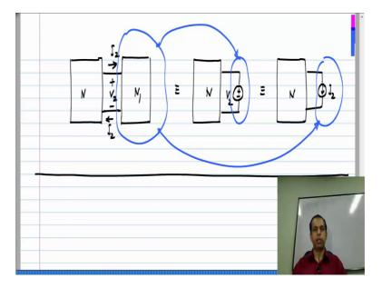
Now, extending this further, let say I had two circuits connected together like this, this circuit I call N and this circuit I call N 1 and they are connected only at two points, that is it. There is no other connection elsewhere in the circuit for this or that one, inside there may be lots of components, but this circuit and that circuit are connected only at these two points and it turns out that, the voltage across this is let say V 2 and the current going that way is I 2.
