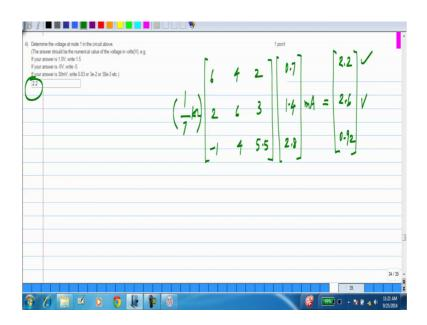
On this problem again refers to the solution of the previous problem, turns out that if you compute the inverse of the G matrix you will get 1 by 7 kilo ohms times these numbers in the matrix and inside you have 0.7, 1.4 and 2.8 milli amperes. Again milli amperes times kilo ohms give you volts and this answer turns out to be, these voltages turn out to be 2.2, 2.6 and 0.92 volts. You are asked for the voltage at node 1, which is that you have 2.2 volts over there.
