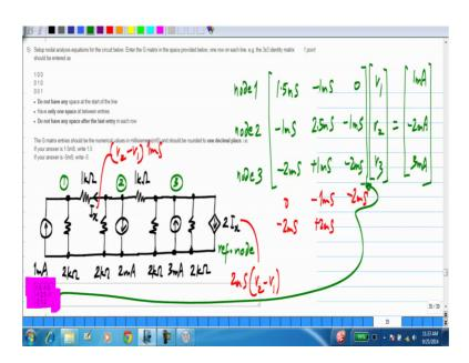
Now, we have again the same circuit different values of current sources and also we have a current control current source instead of a voltage controlled current source as in the previous problem. Now, this is connected to node 3, so it will only effect the equation for node 3, we can write the once for nodes 1 and 2 as before by looking at the sum of conductance's and conductance's connected to the other nodes, the circuit is the same. So, the first two rows will remain the same.
