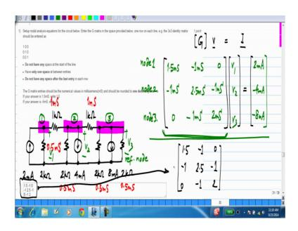
Now, the first question here you are given a circuit and ask to determine the conductance matrix for the nodal analysis. So, this is the easiest of cases for nodal analysis, we have only resistors and independent current sources and there are four nodes as you can see and the reference node is already given to you. These nodes are numbered 1, 2, 3; this is so that you put the entries in the right order and it is easy for us to check answers.
