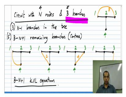
We have a circuit with N nodes and B branches and circuit with N nodes will have N
