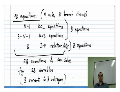
So, earlier we said that we have to solve for 2 B variables. Now let us see how we get the 2 B equations, where do we get them from first of all we have N minus 1 KCL equations. So, this is for an N node, B branch circuit. So, N minus 1 KCL equations, B minus N plus 1 KVL equations, and these two together will give us B equations. And also we have B branches, so each branch will have its current voltage relationship. So, we have B I-V
