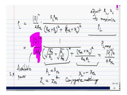
So, the power delivered to the load is mod V square by 2 real part of Z L which is R L and modulus of Z L plus Z th square, which is R th plus R L square plus X th plus X L square. And I have to adjust R L and X L to maximize P L. So, what are the conditions? Quickly.
