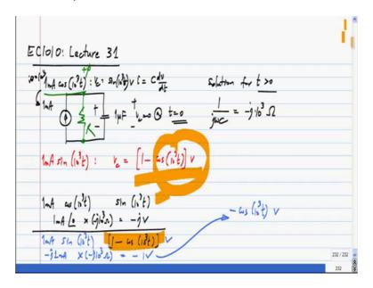
In the previous class we learned how to do analysis of circuits with phasors, phasors are this complex multiples of exponential geometry and from that you can get the sinusoidals study state response. So, I looked all lines and simple compared to solving differential equations, but we did running to a problem, but this particular circuit. So, we calculated it in the time domain we got something and we calculated using phasors and we got something else.
