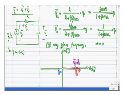
So, now, let us go back to our simple circuit and let say here I apply V p angle 0, what this really means is in the time domain I have applied V p cos omega t. So, now, what is V R and what is V c what is V R, so this is R by j omega C times V p, which is the same as j omega C R by 1 plus j omega C R times V p and this V c is the compliment of that, which is basically.
