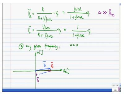
So, now, you should be able to quickly tell me what happens at very high frequency and again high frequency meaning omega much more than 1 by R C. So, this 1 by R C is some characteristic frequency of this this network, because you see that its omega time C R that matters whether omega time C R is much more than 1 or much less than 1 tells you the behavior of each of these phasors there are some question, which 1 V of.
