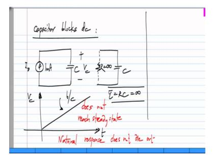
Now, this can sometimes get very confusing, because what if I make a circuit like this let say this is a 1 milli amp current a constant current and I just connected it into a capacitor. So, clearly by Kirchhoff current law this current has to be flowing through a capacitor and so what happened to this statement that d c cannot flow through a capacitor here d c is very much flowing through a capacitor.
