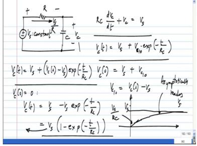
1 0 exponential minus t by R c and let us say the initial value on the capacitor was some V c 0 or may be V c of 0. So, what is the value of V c 1 0? So, V c of maybe I think this will again... If I substitute t equal to 0, V c of 0 should be V s plus V c 1 0. So, V c of 0 minus V s is the, this constant V s plus V c 1 0 at t equal to 0. So, the; obviously, V c 1 0 is V c of 0 minus V s. So, this V c of t can be written as V s plus V c of 0 minus V s exponential minus t by R c.
