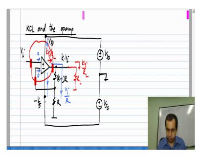
Let me take our usual amplifier circuit, if I have an input voltage V i and this is k minus 1 R and R, the output will be k times V i with an ideal op amp and with a real op amp for the finite, but very large gain, it will be close to this. Now, the current flowing through these resistors is V i by R, it is k V i divided by the sum of these which is V i by R. Alternatively V i appears here also, so the current through this is V i by R which also flows through that resistor.
