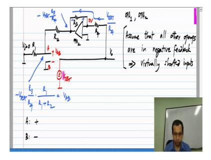
So, let me first determine the sign OPA 1 and then OPA 2 the ordering has some influence as we will see later and V i set to 0 which means that this is connected to ground we are determining the signs of OPA 1; that means, that this is removed and I apply V test here let me call these A and B and I will determine V A B over there. Now, the rest of it is regular circuit analysis, the only thing is this what to do about of the other op amp.
