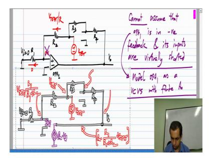
We have to determine the signs for OPA 2. So, the signs for this op amp have been determined as plus and minus and V i is 0 which means this is grounded. Now, I will remove the second op amp and apply a test voltage like that. Now, what to do with OAP 1, we can try the same assumption that is that OPA 1 would be in negative feedback. So, it is inputs are virtually shorted, but now we will run into a contradiction, because let us assume that the inputs of OPA 1 are virtually shorted.
