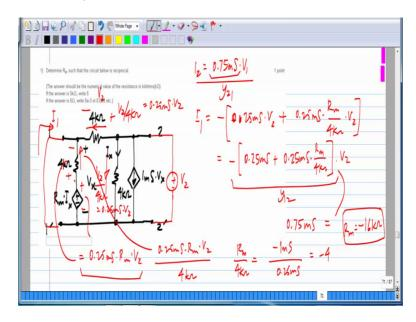
The first question is about a two port network consisting of controlled sources, this means that the network is not necessarily reciprocal, but for certain parameters of the controlled sources it can be reciprocal. The question is to find the value R m; such that it is reciprocal. So, all we have to do is find the two port parameters and specifically we have to find only y 2 1 and y 1 2 or any of the 1 2 1 2 parameters to check for reciprocity.
