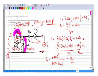
Now, this is another network with controlled sources and you have to find the value of the control source G m; such that the network is reciprocal. In this case you can choose any parameter set, let me choose z parameters. I have to find z 1 2 and z 2 1 and make them to be equal to each other. So, first I will apply I 1 and measure V 2 with port 2 open circuited, they should give me z 2 1. Now, with port 2 open circuited the current in this branch is 0, so V x is 0, so this just goes away.
