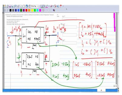
Finally, this question here is it shows to 2 port network connected in some way and you can easily see that they are connected in parallel and h parameters are given for one and G parameters are given for the other one and you should find the y parameters of the combined network. Now, if I call this I 1 A and I 1 B and let me call this V 1 and I 1 the voltage applied to port 1 of the first two port as V 1 second two port is also V 1.
