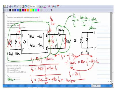
So, we have this current source open circuited the voltage source short circuited and we can find the resistance in here whatever resistance we find that parallel with 10 kilo ohms, because 10 kilo ohms appears directly across 115 is the net Norton resistance and this one again we write the 2 port equations. So, let say this is I 2 and this is V 2. So, the resistance looking then there would be V 2 by I 2 and let say this is V 1 and that is I 1.
