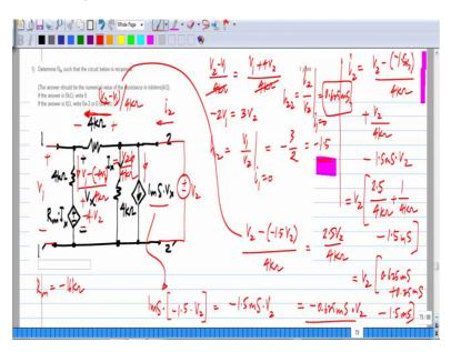
Now, for two more parameters we have to apply a voltage to the second port with the first port left open circuited. So, if you apply V 2 here, this I x will be V 2 by 4 kilo ohms and this R m I x we determined R m to be minus 16 kilo ohms. So, this R m times I x will be minus 4 times V 2. So, now, we have to find V 1, we know that the current flowing this way is V 2 minus V 1 divided by 4 kilo ohms and the current flowing that
