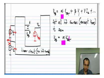
So, to do that let me do the following, I will remove the op amp. So, this was terminal A, this is terminal B, like I said we have to find out what fraction of voltage applied here comes back to it is inputs and let me apply some V tests, where the op amps output was, so this is the first step. So, if you look at the original circuit, the op amps output is here, now what I did was I removed the op amp and wherever the op amps output was I now drive it with some test voltage V test.
