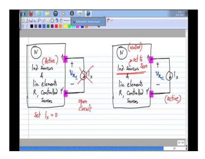
So, first what I will do inside the independent sources will be active and I will set I x to zero, so when I set I x to 0, what happens this is an open circuit and in the next case this I x will be active and this independent sources. Any number of independent sources inside will all be set to 0 and this is known as nulling the circuit. So, I have nulled the networking that means any independent sources I have set to 0, but I x is active, so I will get let us say call this V x 1.
