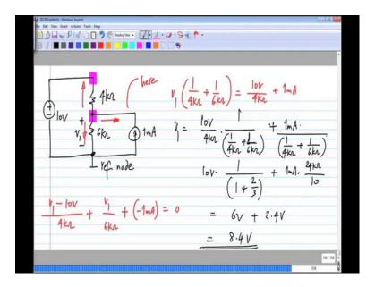
So, V 1will be 10 volt by 4 kilo ohm, 1 by 1 over 4 kilo ohm plus 1 by 6 kilo ohms plus 1 milli ampere divided by 1 by 4 kilo ohms plus 1 by 6 kilo ohms. So, if I take this inside, I will get 10 volt 1 divided by 4 kilo ohm this gives me 1 plus 4 by 6, this gives me two- thirds and this one here if I calculate this I will get 6 kilo ohm plus 4 kilo ohms divided by 4 kilo ohms. This is basically 10 by 24 kilo ohm in the denominator we have kilo ohm square in the numerator, we have kilo ohm.
