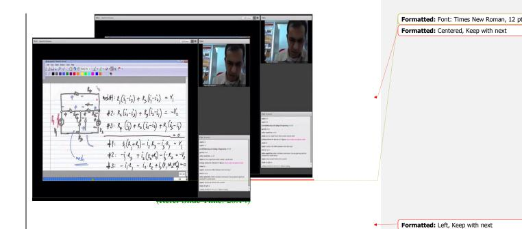
So, I will have i 1 r 1, plus r 3 minus i 2 times r 3, minus i 3 times r 1 to be equal to v 1 that is the equation for mesh number 1 and equation for mesh number  $2_i$  that is minus i 1 times r 3, plus i 2 times r 2, plus r 3, minus i 3 times r 2, that will be minus v 2. And similarly, for 3 will have minus i 1 times r 1, minus i 2 times r 2, plus i 3 times r 1, plus r 2 plus r 4 equals 0.
