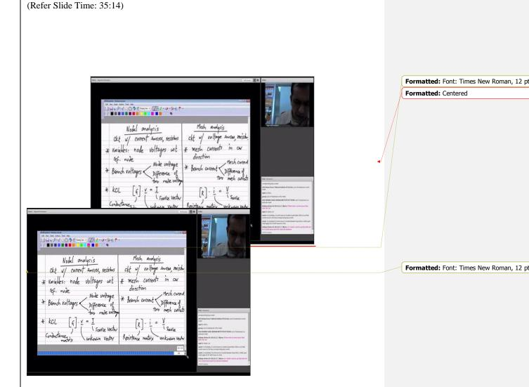
Now, you can see the analogy with the Nodal analysis very easily so first of all, I will compare Nodal analysis of a circuit having current sources and resistors versus Mesh analysis which of a circuit with voltage sources and resistors. Now, in case of Nodal analysisanalysis, the variables are node voltages with respect to reference node and in case of Mesh analysis the variables would be mesh currents in clockwise direction.
