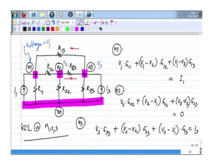
Now, a KCL at node n 1 will be the sum of these currents current through r 1 1 current through r 1 2 current through r 1 3 the sum of those equal the current flowing into this node which is I 1. So, first of all the current through r 1 1 is V 1 divided by r 1 2 or V 1
