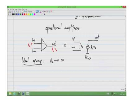
Now, what is an operational amplifier? It is just a voltage controlled voltage source and because it is a block, that used so often it has a symbol of its own which is given by this, this is clearly equivalent to... I will call this in p for positive inputs, and in m for negative input and output, this is equivalent to in p and in m and a voltage controlled voltage source. What does the voltage controlled voltage source give out, it gives a
