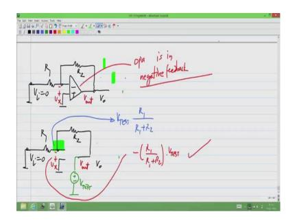
Again, we can apply the same algorithm, so first I null the input that means that I short this to ground that is V i equal to 0, so then I remove the op amp apply V test, sorry I also had to identify let me remove this before coming to this step. I had to identify the input voltage V x and the output voltage V out of the op amp, then I remove the op amp and apply V test to the output of the op amp.
