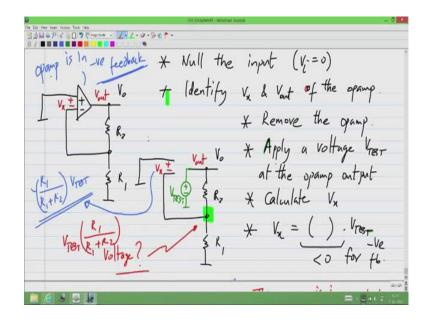
You null the input because this is nothing to with input feedback refers to what fraction of the op amp output comes back to its own input identify V x and V out of the op amp whichever op amp you want to find the feedback. Then, you remove the op amp in place of the op amp's output you apply a test voltage V test and then now you have a basic linear circuit which you can analyze and find the input the input voltage V x of the op amp.
