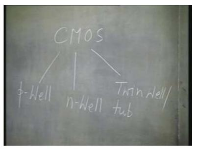
So, we can have in CMOS technology, either a p-well or an n-well or better still, we can start with a very low doped substrate material, nearly intrinsic and we can have both the wells, which is called the twin well or twin tub technology; twin well or twin tub. These are the three different ways in which a CMOS can be realized.
