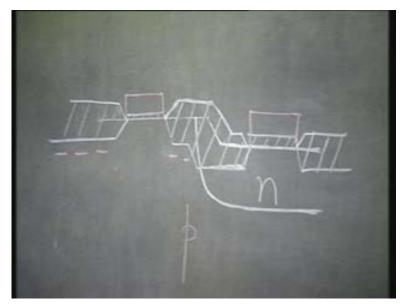
So, now underneath this you have boron implantation; may be I should just show it with dots and now I can remove this silicon nitride-oxide mask.
