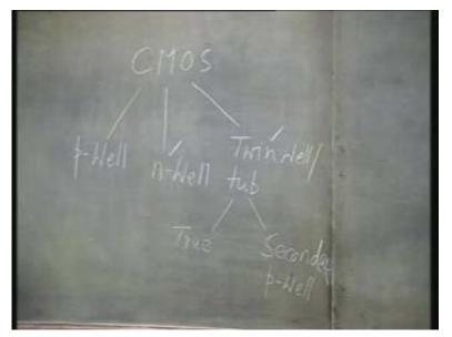
Now, as far as the CMOS technology is concerned, these two are the most important techniques today. Previously, because n MOS was the dominating device, the most widely used MOSFET we used n-well technology, which was compatible with the n MOS process flow and now as CMOS itself has become the dominating device in VLSI, now we use twin tub or twin well technology. So, let us first discuss the n-well technology, how exactly the well is created and then we go over to the twin well technology.
