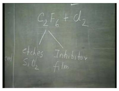
One job is it etches silicon dioxide, the native oxide that is always present on any silicon surface and secondly, it forms inhibitor film, so that you get very good anisotropy even when you are etching heavily n-type silicon.
