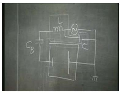
As you can already see here, usually in a plasma reactor we have a permanently grounded electrode, which we call the anode. So, therefore that anode is always at zero potential, right. If we have an insulating surface immersed in the plasma, then it is going to acquire a small negative potential which is called the floating potential and this is the floating potential.
