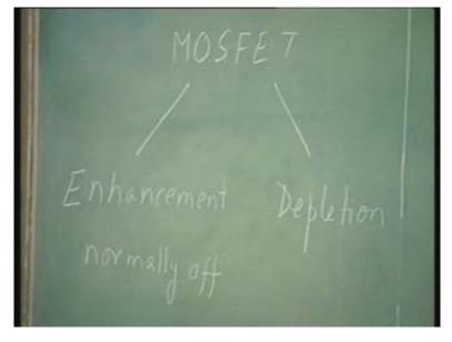
Enhancement mode MOSFET are normally OFF MOSFET, depletion type MOSFET are normally ON MOSFET. What do I mean by these terms? I mean that if it is an enhancement mode that is normally OFF, which means when no gate voltage is applied this MOSFET is not conducting, this MOSFET is OFF. I have to apply a gate voltage in order to make the MOSFET conduct. In contrast, a depletion mode MOSFET is conducting when no gate voltage is applied and I have to apply a gate voltage in order to switch it OFF.
