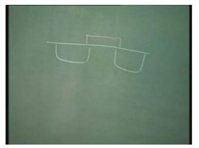
If I have my source here and drain here, then the gate oxide must extend from here to here. It should not be shorter than this. For example, it should not be like this.
