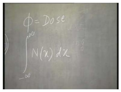
So, the dose which is called phi, in ion implantation this is the notation which is usually used, that is the dose that is given by ...., simply by integrating it between the limits minus infinity to plus infinity. Now, you already know what N(x) is. Let us try to integrate this. So, what do we get?
