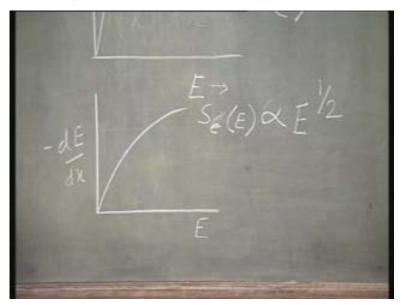
On the other hand, if you look at the electronic stopping, this increases like this. That is S e, it is proportional to the square root of energy. So, you see at the starting point where the ion is just penetrating the semiconductor, the electronic stopping is highest and then, as the ion starts losing its energy, the electronic stopping becomes less and less.
