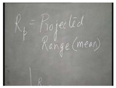
So, this is actually the projected range, mean value of that and the variation in the projected range will be taken into account by a factor delta R p, which is actually the standard deviation in statistical parlance and in ion implantation jargon, we call it the straggle.
