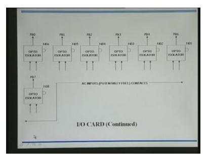
Here are the seven circuits for opto-isolated inputs. It is potentially free contact for various parameters that we need to measure, which we have already seen earlier as temperature high and so on. There are seven.
