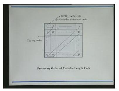
The DCTQ is actually created in raster scan order as 1, 2, 3, 8, then 9 and so on. This is per block – per block is eight by eight pixels. In VLC, you have to code in this fashion: 1, 2, then 9, then go on to 17, then 10 and so on. It goes diagonally and it is called zigzag order and right up to 64. This is for the variable length code processing.
