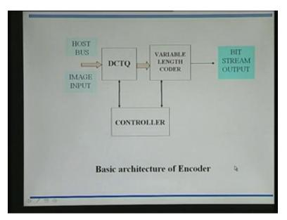
What all you have to do is you need to design the variable length decoder before you output the DCTQ output on to the stream. You also need to have a controller at the encoder end.
