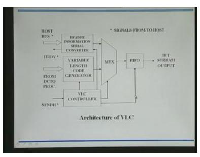
The block diagram for the variable length coder is here. This is the main unit wherein DCTQ is fed and each of the coefficients is translated into a variable bit. At the lowest end, it will be two bits and at the highest end, 28 bits. Finally, all said and done, you get a compressed bit stream here. You need a FIFO so that you accumulate first all the bits and then finally transmit in a controlled manner.
