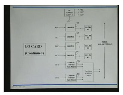
The I/O card also has four relays at the output and there are drivers. These ports are the ones that we will have to connect to the FPGA board and the power supply is shown here.
