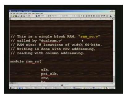
This is another file and this file is being called by dual RAM that is what is indicated here. RAM size is as you know eight locations of width 64-bits and writing is done with row addressing reading with column addressing. This also we have covered for dual RAM, same thing applies for RAM\_rc and once again the I/O details are exactly the same as we have seen before.
