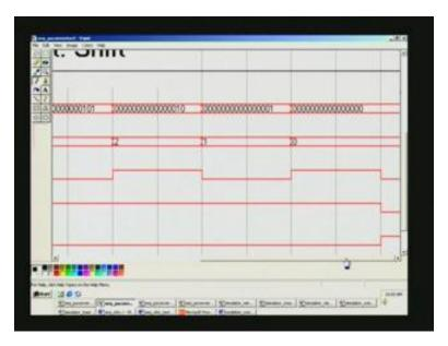
Now you can see after this is over that all these transactions are taking place at the positive edge of the clock. You can just see here. It happens every time, as you can see the positive edge here and positive edge here. Finally, an end of conversion is asserted here. This is the last for the data therefore data valid goes low.
