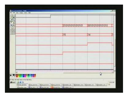
0 is first here, then 1 here. Hereafter, it should be 0 1 and so on, in a toggling mode. This is the very first waveform we already had a look into. The second one which we did not have last time is this and this is towards the end of the right shift.
