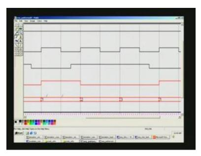
Now, one has come, so again you see two 1s are there, even when the last pattern is taken into account. 0 1 1, once again you see a 0 here, so promptly goes to the output high here and from third state you should finally have seen here. It should go to one state, provided this input is 0 in third state it is here. If input is 0 it should go to one state output is 1. That is what we have here.
