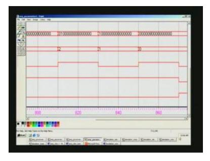
We started with 0 1 0 1 etc. so the very last must be 1 because it is a left shift; 0 1 0 1 0 1, so the last bit will be 1 and after it shifts here and once again data valid goes low and end of conversion is activated here. This completes the parallel to serial converter and will go on to state machine.
