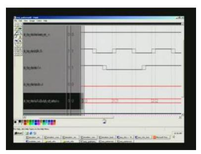
Here, the actual input is applied little offset, as you can see. This is because when we come to positive edge of the clock it must see stable value at the input.
