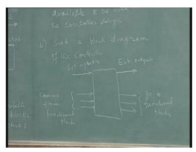
Having done this I take into account the operational requirement we have only designed the functional blocks. We have not talked about how to carry out the design operation required to be performed by the functional unit. This will be represented by this will be explained or this will be described by means of a procedure. I need to draw a procedure of control you see here for the controller operation actually.
