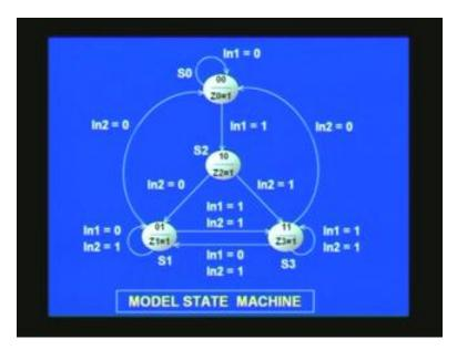
Next we will consider how to model a state machine. Let us say we have 4 state machines and in each of these states you wish to light up an LED or a lamp. Zee stands for one lamp; zee 0 stands for the s not condition state indicator. If you are in s not state, then this lamp will glow and likewise in all other states and this s not is the state and in binary notation. Let us say it is 0 0.
