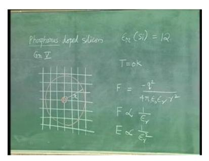
Phosphorus doped silicon: The phosphorus is a group 5 element. So whatever we discuss now is applicable to group 5 impurities in general. If you introduce phosphorus impurities in silicon what is the picture? Let us draw the bond model of pure silicon first; that is a two dimensional matrix and we assume that in this matrix somewhere instead of silicon you have introduced a phosphorus atom.
