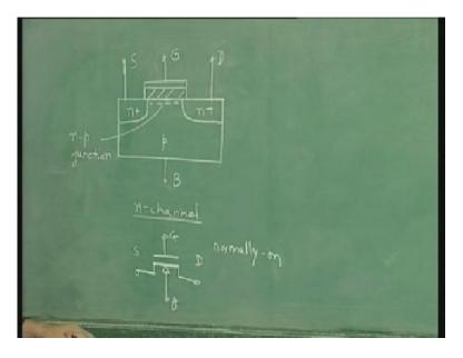
Let us look at this structure of an n-channel device and correlate the structure to the symbol. So you have the gate then you have the channel. Now, if this is a normally-off device then the channel will not be connected between source and drain when there is no gate source voltage and in such a case the channel is shown by dotted line. So if the channel is shown by dotted line it is a normally-off device. Now you have this source and drain terminals, this is the gate, source and drain.
