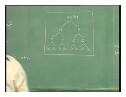
This is the MOSFET, you can have either n-type or p-type. Each of these can be enhancement or depletion and each of these devices further can be either surface channel or buried channel. So these are all the different types of MOSFETs we have. Having discussed the various types of devices and broadly seen the device structure let us understand the symbol of MOSFET also now.
