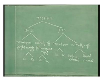
So, MOSFETs can be n-channel or p-channel and further each of these devices can be normally-on or normally-off. This normally-on device is also referred to as depletion-type device while the normally-off device is referred to as enhancement type device. Now let us understand the meaning of these terms normally-on and normally-off. For this purpose let us look at the device structure and its operation in a little bit more detail.
