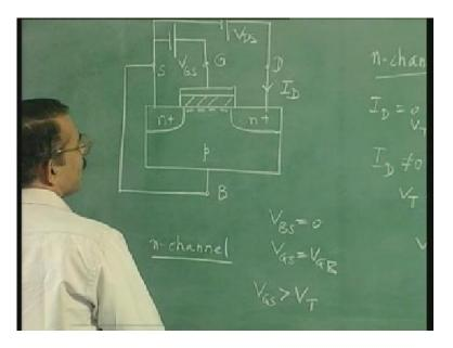
So this is an n-channel MOSFET. Let us name the various terminals here, this is the gate, this is the substrate. Now we shall call the substrate as the bulk. The reason is substrate and the source both have letter starting with s. So when you use symbols with the starting letter to denote the particular terminal there will be confusion between substrate and source because both have (s) as the starting letters. Therefore we use the word bulk to represent the substrate. So B stands for Bulk.
