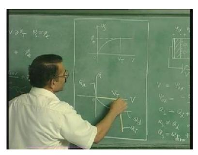
Beyond threshold it saturates to a value  $phi_t$ . This saturation is approximate of course whereas this  $psi_{ox}$  keeps increasing continuously because the silicon charge as a whole which is the sum of the inversion charge and depletion charge keeps increasing though the depletion charge saturates beyond threshold. Now we also derived an expression for  $V_T$  as well as this  $phi_t$ .
