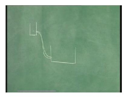
So even if you have a container like this which is small and you have big container here at a lower height than this and when you join these two by a tube the water will flow from this to this even though the container is small because it is at a greater height than here. So it is the height that decides the transfer of water. Similarly here it is a Fermi-level that decides the direction of transfer of electrons.
