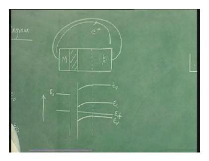
So when a Fermi-level moves up it means that you are applying a negative voltage. So in order to get Flat-band condition what you will have to do is, you have to introduce a power supply here with a negative polarity because in this particular case you have negative charge in the semiconductor.
