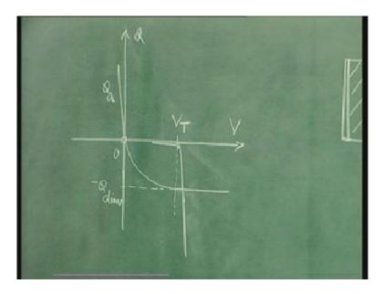
This is the Q versus V curve. For the various segments the equations are as follows. For this accumulation segment that is this segment here you can write  $Q_a$  is equal to minus  $C_0$  into V that is this segment. Then for the depletion segment that is between 0 and  $V_T$  you can write V is equal to minus  $Q_d$  by  $C_0$  plus  $Q_d$  square by 2q epsilon<sub>s</sub> N<sub>a</sub>.
