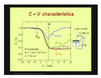
We are coming closer to this explanation. As a first step we said we will explain the charge conditions in the MOS capacitor as a function of the DC applied voltage and from there we will derive the C - V characteristics.
