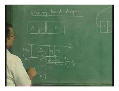
Now let us look at the energy band diagram when all the components of the MOS capacitor are isolated. That means you have the metal then you have the oxide and you have the semiconductor and suppose these are all isolated now without any loss of generality we will assume that the metal is also sufficiently thick, this is just to enable us to draw the energy band diagram.
