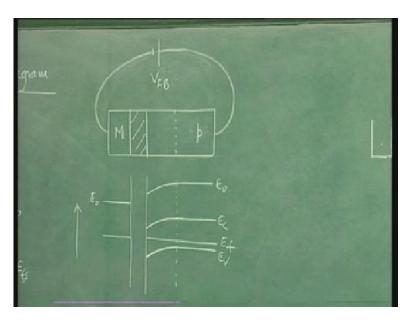
Once you do that provided the power supplies of copper magnitude all these negative charges will be repelled. We will shortly see what the magnitude is. This is interesting that you have zero charge condition in the metal for a given applied voltage so this is the Flat-band voltage. Now V is equal to  $V_{FB}$  is the condition.
