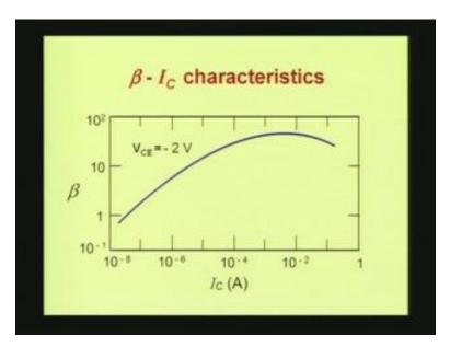
So, the range of the collector current is from 10 to the power minus 8 amperes to 1 ampere here which is a very wide range and that is why the axis is logarithmic. The variation of beta on the other hand can be seen to be from about 1 to a peak of somewhere about 70 to 80 and then there is a fall.
