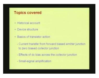
First we looked at the historical account of how this device came into being, then we discuss the device structure. Then we idealized this structure and using this idealized structure we discuss the basics of transistor action. We discussed how the current transistor occurs from forward bias emitter junction to zero bias collector junction.
