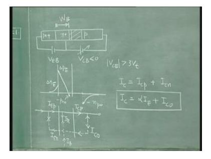
Now the current across this reverse bias junction will also be due to some small amount of holes on this side, this is shown by the fact that this hole concentration has reduced a little bit. But we can neglect this effect because minority carrier concentration on the collector is much more than that in the base so we neglect that effect.
