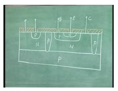
So I can have a diode like this and then I can have a transistor, so this is an example where I am showing a diode and a transistor in the same silicon wafer. This is the so called emitter contact, this is the so called base contact and this is the so called collector contact and they are all in the same plane.
