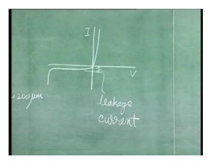
Here are the diode characteristics, this is current versus voltage. So in reverse characteristics this represents the leakage current. That leakage current was high for these devices. Now let us look at the structure of the diode which is made by the Planar process.
