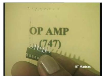
So, two plus one - three plus two - five terminals essentially; and if there are two such op amps, we will have ten terminals taken care of. And in this fourteenth pin, we have possibility of what is called offset compensation, about which we have also discussed. So, two terminals for one op amp and two terminals for the other op amp for offset compensation. So that forms the fourteen pin base and the base diagram we can see here; top view of L M 747.
