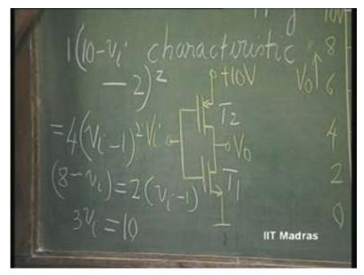
So, V i equals how much is it? 10 by 3. Is this clear? So, this is 10 by 3 is 3 point 33, so on...
