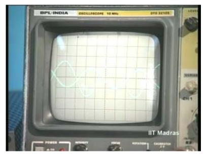
So, this is depicted there on the oscilloscope. If you couple it along with the scale given, you will see that the gain is exactly equal to 250. Further, we will check the operating points. Now, Padmavathy will show us using a D C multimeter, the potential at the base which should be 2 point 84.
