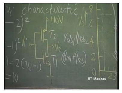
So, these two amplifiers are working in parallel on to a common load which is r d s 1 parallel r d s 2. Since they are working in parallel, the effective g m will be g m 1 plus g m 2 into V i. So, we have understood how this can be used as an inverting amplifier with this kind of gain; how it can used as a digital inverter; and we also know how this current varies with respect to what? – signal, V i.
