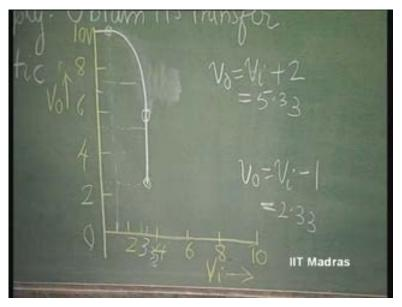
So, this region from 2 point 33 to 5 point 33 - for a region of 3 volts, which is strictly speaking, magnitude of V T N plus magnitude of V T P; 1 plus 2, 3 volts here, it is having infinite slope; thereafter, up to 8 volts... What is 8 volts? 10 minus magnitude of V T P; 10 minus 2 volts - 8 volts. This story will go on. After this, transistor T 2 will go off.
