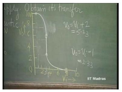
So, this is the complete characteristic of our CMOS inverter where, if you draw a 45 degree line... 45 degree line, what is the slope? Tan 45. That is minus 1 here. You can draw a similar line here. It is within this region that we say that the transistor, CMOS inverter, is in the active region; gain is greater than 1. Beyond this region, it is not in the active region. It has gone into what? One of the two saturation stages: either this or the other one.
