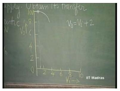
So, the other line is V naught equal to V i minus 1, corresponding to this transistor going to triode region. Again, it is this V D S, which is V naught itself, is equal to V i minus 1. That is the region where it is entering the triode region. Now, in between, we have both transistors in current saturation region. Therefore, we have K P which is 1 into... now, this is important; V G S minus V T, which we are going to always refer as V S G. So, 10 minus V i minus 2 volts.
