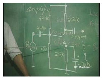
And then, we have the potential at the collector. Once again, she will now connect, connect it to the collector terminal which should be around 8 point 8 volts D C potential. So, you have that voltage 8 point 68 which is pretty close to 8 point 7 volts, which is pretty close to the expected value.
