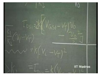
So, this is the equation that is going to be valid and V G S 1 is equal to v i. So now, you will see I D S 2 is going to remain the same. Only I D S 1 is going to change. Again, I D S 1 is equal to I D S 2. Now, this is no longer linear. This is nonlinear because you have square, linear and square here.
