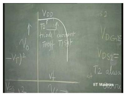
This is going to be the case, as long as this particular thing is going to remain in the current saturation region. A point will reach when this transistor will enter the triode region. This is going to enter the triode region. So, this is going to go on until the transistor enters the triode region.
