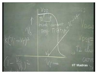
So, this is the advantage of this scheme. When the both, this and this, are in the triode region, we have this acting as a high gain amplifier. So the slope is going to be infinity and the transition is going to take place like this. Unlike this situation where the slope depends upon the K 1 by K 2 ratio, here, we have the slope becoming equal to infinity.
