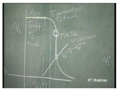
I would like you to evaluate the transfer characteristic for this portion where the entire amplifier is in saturation; equating the...for T 1, current in the triode region to the T 2, current in the saturation. That is of course I D S S.
