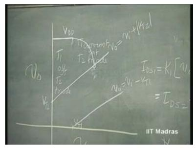
That means this equation is no longer valid. I D S 1 equal to I D S 2. This is equal to T 1 and T 2 in current saturation region; and therefore it is going to be infinite gain; slope is going to be infinity.
