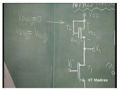
Now, this is V D S 2, this is V G S 2. And V D G 2 equal to zero. Therefore, V D S 2 has been made equal to V G S 2 in this case. So, what is the state of affairs as far as the T 2 is concerned? T 2 therefore is always in current saturation region. Why? Current saturation region, a transistor is going to be, as long as V D S is greater than or equal to V G S minus V T.
