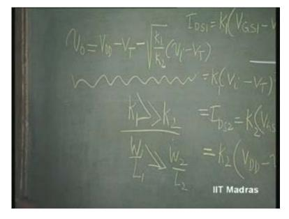
So, this is the design aspect. So, if we make them identical, then it will be having unity gain which is not good, either for amplification or for inversion, inverter application, in the case of the digital circuit. So, this is always what is done.
