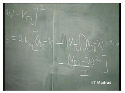
So, there is not going to be any confusion here. Otherwise, you stick to the original equation with signs being properly taken care of. So, this equation will give you some kind of non-linearity here. Up to a point, this will go on. The triode region, T 2 remains, until a point is reached at which it will come into current saturation; that we have to find out.
