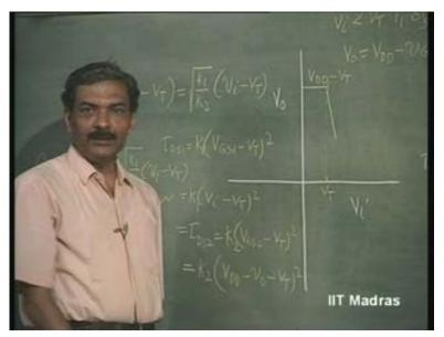
For a good inverter, we have mentioned that this slope is nothing but what is it? - the gain of the amplifier in the active region. The slope is nothing but the gain of the amplifier in the active region. This should be both in the digital inverter as well as amplifier, very high. That means K 1 should be much greater than K 2. Or, W by L ratio of transistor 1 should be much greater than W by L ratio of transistor 2. Is this clear or not?
