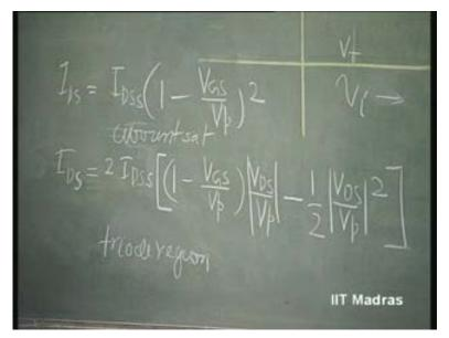
Now, this current is going to be equal to this current, I D S 2. V G S in this case is zero at all times. So, this is zero. This into V D S minus V P. That is all. 1 into V D S minus V P.
