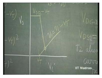
So, that I am going to leave it as an exercise for you. Solve these two equations and obtain V naught and V i at this point, the transition. Thereafter, this equation is going to change because it has entered the triode region. I D S 1 is no longer K 1 into V G S 1 minus V T whole square. It is equal to what? 2 K 1 into V G S 1 minus V T into V D S, which is V naught, minus V naught square by 2, V D S square by 2.
