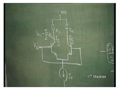
So, this kind of thing can be prevented if you take care to see that this common mode voltage does not exceed this here. On the other side, this voltage can go down and this voltage will follow this. V c minus V Gamma will be the voltage here. And at that time, this current source should remain still active. So, that is the condition. So, there is a limit on V c max as well as V c minimum, as far as the input stage is concerned.
