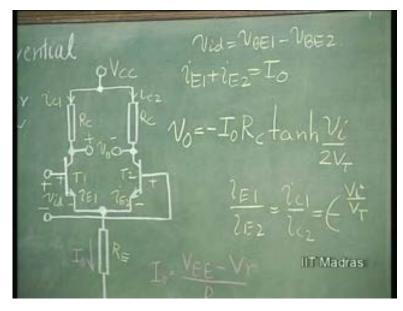
And then we saw that i E 1 by i E 2 ratio is exponent V i by V T, from which we derived V naught as equal to minus I naught R C tan hyperbolic V i by 2 V T, I naught being equal to V E E minus V Gamma by R E. Then we said we will plot this; and this plot tells us that for V i negative, output is going to be positive; V i negative... This is going to be minus 1 and there is minus 1 here; so, it is positive I naught R C.
