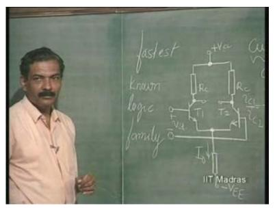
Why is it fastest compared to other logic families? When the current is completely switched to this, the potential here is V C C minus I naught R C. At that point of time, T 1 should not go to saturation. That means there should be enough collector to base potential, which is positive in this case, in order to retain T 1 in active region. This is an important aspect.
