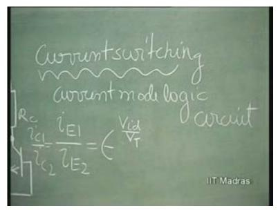
So, a differential amplifier is belonging to a family of logic circuits called current mode logic circuit; or, it is in this particular case popularly called emitter coupled. Emitter is coupling this transistor. It is coupled at the emitters to a common point. So, this is called Emitter Coupled Logic or popularly, E C L; or, Current Mode Logic, E C L or C M L, current mode logic.
