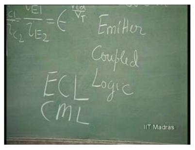
This by nature, because only the current is switched from this to this; by nature, is the fastest known logic family resulting in... Any computer designed using this logic family will be the fastest computer run. As far as transistors are concerned, any computer using such logic family is going to be the fastest logic family computer; and therefore fastest computer.
