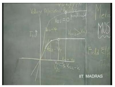
So, this is called pinch off. So, this is called the F E T action. What is FET action? Causing it to pinch off and letting the current go to saturation. That will happen corresponding to V D S greater than V G S minus V T. Therefore, transistor is said to be in current saturation region.
