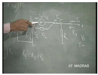
This current is Alpha times i e; and I know the current in this. Alpha times i e has to be subtracted from the total current which is i e plus i e r e R B dash. Then, that will be the current in r c. This current is i e plus, i e plus i e r e by R B dash. From this total current, I subtract this Alpha times i e. That will be the current through r c. Now, once I know the current through r c, drop across this is, that current into r c.
