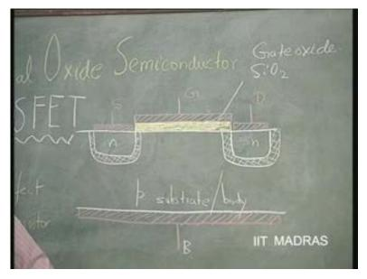
Why it is made thin is because we would like to have control over a surface by the gate electrode. So, you would like to make it as thin as possible so that the control is good. What does the voltage apply to the gate too with respect to the substrate, we will see that.
