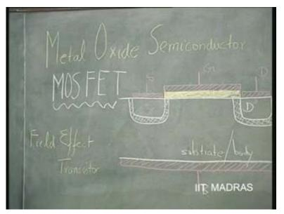
So, this important device is called Metal Oxide Semiconductor Field Effect Transistor, Metal Oxide Semiconductor Field Effect Transistor, which is abbreviated as popularly M O S FET; F E T, MOSFET. It is necessary that we understand this active device in the same way we understood bipolar junction transistor. So, I will now discuss qualitatively the characteristics of MOSFET. This is the backbone of all our MOSFET circuitry discussion.
