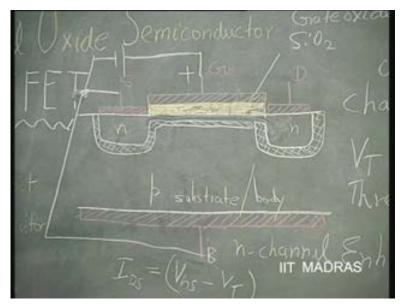
So, this voltage is zero. Now, I am applying a voltage V G S between gate and source. So, the current is going to depend upon V G S minus V T. V G S, if it is equal to V T, current is zero. It is completely blocked. There is no channel formulation. The channel formulation occurs only after V G S equal to V T occurs. Substantial amount of current can now flow. So, the current is dependent upon the factor V G S minus V T; so, dependent proportional, initially.
