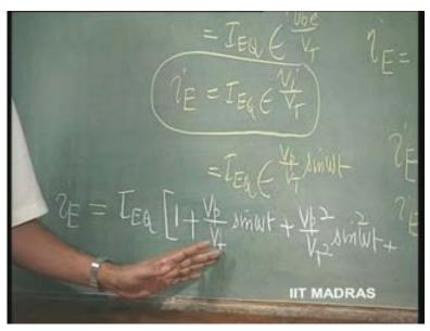
So, there is i E superimposed over I E Q plus I E Q by V T into V p sine omega t; this is the input voltage. So, this I E Q by V T into V p sine omega t is the factor of importance in an amplifier, linear. The other part is, let us see, V p square by V T square into... sine square omega t can be expanded as 1 minus cos 2 omega t by 2. So , ignoring the other higher harmonic factors, because there will be factorial x square by factorial 2 t and x cube by factorial 3, which is 6, so on...
