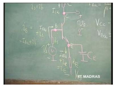
Now, when this happens, what will happen here? I E Q will be I E Q plus, the change that has been brought about, that is i small e, which is really the i instantaneous. So, for a change in signal voltage here, because base to emitter current, voltage, increases, correspondingly, emitter current increases, the base current increases; you can think of it that way. Then, corresponding to this, we will have a change in collector current, which will result in the instantaneous value.
