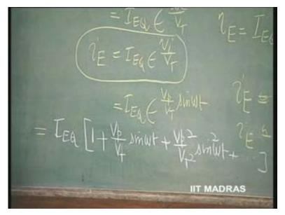
This, we had derived in the earlier situation also. This is what is wanted. Actually, if I want the instantaneous value of the emitter current to be linear with the input voltage which is V p sine omega t, linearly related; I want these factors to be very small compared to this factor.
