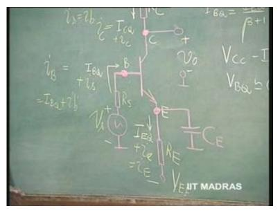
All these can be assumed to be linear relationship. That is, that I C Q equal to Alpha times I E Q is valid; and Delta I C Q is equal to Alpha times Delta I E Q is valid, assuming that Alpha A C is very nearly the same as Alpha D C. Then, the change, for change in signal also, this same relationship is valid.
