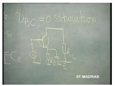
Now, the transistor can be replaced by its equivalent circuit, linear equivalent circuit, where you are going to replace this by small r e; and this by Alpha times i e, when this current is.... All these directions, you must definitely put. This is valid all for...only this signal, i s. So, v s is kept as such, r s is kept as such; and through this v s r s combination, instead of I B Q plus i s flowing now, only i s will flow. So, through this, only small i s will flow.
