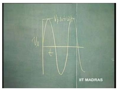
So, if v s is V p sine omega t, then, if the base to emitter change is very small, the change in voltage is very small, corresponding to which there is going to be a change in emitter current. That is, Delta V B E and Delta I E which are now being replaced by Delta i e; is replaced by i e, small suffix e.
