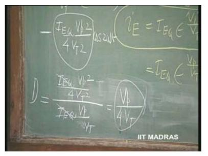
It is an important thing; quickly you can assess now, the amount of distortion in a common emitter amplifier if your input voltage is given as, let us say, 1 millivolt, let us say peak; V p is given as 1 millivolt, peak, 1 millivolt sine omega t, let us say. Then, this will be 1 by 4 into 26 millivolts. If you want for assessment, you can take V T as 25. So, 1 percent distortion is what is going to be caused for a signal of 1 millivolt.
