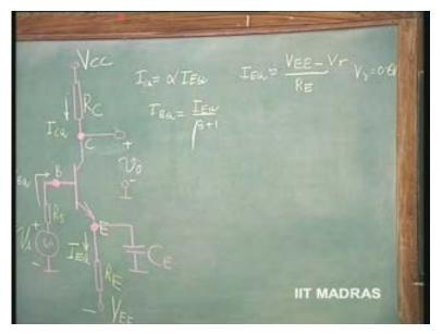
So, this is what we had biased the transistor at. The voltages V C C minus I C Q R C is equal to V C, with respect to ground; and V B, V C Q we will put it, V B Q is very nearly zero. This is what we said. Because, it is equal to I B Q into R S with a negative sign, minus I B Q into R S.
