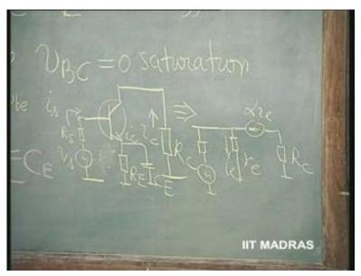
Now, V C C is grounded; and instead of through this now, I C Q plus i c flowing, only i c will flow. Instead of through this, actually speaking, we will put it here, i e will flow. And this i e will flow, not through this r e, but through this capacitor which is a short circuit.
