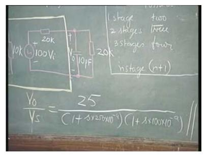
Now, I would like to expand here. Suppose we plot the Bode's plot. Then, this corresponds to gain of 25, remaining constant. If you convert it into decibels, it will be 20 log to the base 10 of 25. That is the decibels. 20 log to the base 10 of 20; whatever it is. That is the gain, constant gain, at low frequencies.
