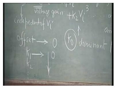
So, we will bias the active device; or, we will select the operating point of the device; or, we will design the circuit, the complex circuit, containing large number of devices, active devices, in such a manner that this whole thing is true. So, design of an amplifier involves selection of the operating point and the bias in such a way as to make the nonlinearities the minimum, linearity the maximum and offset voltage the minimum.
