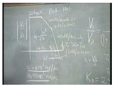
How do you evaluate this? This is very simple. Upper cut-off frequency, we have also said, is nothing but 3 dB point, upper 3 dB point, where the gain falls to 1 over root 2 times the maximum, the low frequency gain. So, if the gain of this is 25 by this, then, when the gain falls to 25 by root 2, that is the frequency corresponding to upper cut-off frequency.
