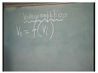
Strictly speaking, in general, any device will give me an output which is a function of V i; not just necessarily proportional to V i. So, if it is a general function of V i, then, that function can be split up as something, let us call it as a voltage, which is going to be called offset. This is independent of the input voltage. This is a voltage which is independent of V i. That voltage is called, as you have already seen, it is called offset voltage.
