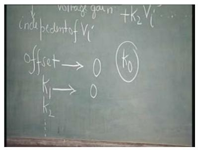
So, K naught is something that should be as stable as possible. Offset should go towards zero; K 1 should go towards zero; K 2 should go towards zero; all the nonlinearities should go towards zero. So, amplifier nonlinearities cause, again, distortion. This has nothing to do with frequency. This has only to do with amplitude of the input signal. So, this distortion, this depends upon where exactly we are operating in the amplifier, so called amplifier.
