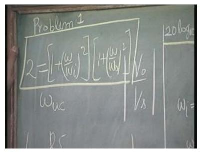
So please, as a homework problem complete this. That is not part of the example problem. Obtain the cupper cut-off frequency for the example. Obtain the upper cut-off frequency for the amplifier. So, you will notice that the upper cut-off frequency is going to be less than the lowest of the corner frequencies.
