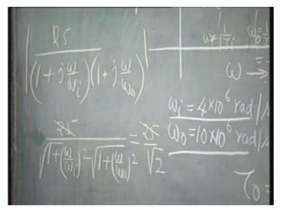
So, we can square this. So, 2 becomes equal to 1 plus omega by omega i whole square into 1 plus omega by omega naught... So, this is going to be a quadratic equation, which if you solve, will give you the upper cut-off frequency. So, I would like you to work this out; solve this quadratic equation. This is a quadratic equation in omega by omega naught, omega square; to get omega to the power 4 and omega square. We can solve for omega square and get the upper cut-off frequency here.
