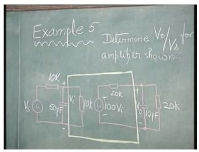
Determine V naught over V s, V naught over V s, that is, the amplifier gain for the amplifier shown, wherein, apart from the usual input impedance, source impedance, output impedance and the load impedance, we have the effect of stray capacitance; one at the output, 10 picofarad, one at the input, 50 picofarad. The input capacitor, total together, comes out to be 50, let us say; and the output capacitor comes out to be 10 picofarads. This is the typical order of the amplifier capacitors.
