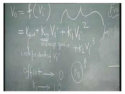
K 1 is zero; K 2 is present. This is going to have this kind of nonlinearity which is symmetric both for positive going and negative going signal, has K 1, K 3, etcetera, going to zero. But, K 2, K 4, etcetera, existing. So, this is one type of nonlinearity; so that depending upon the device that you select, the nonlinearities will change.
