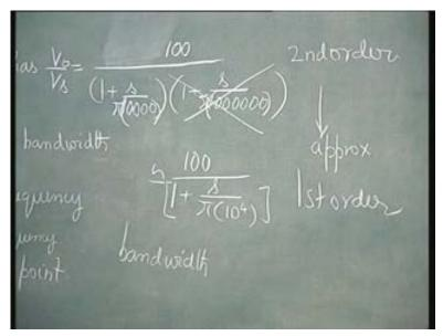
So, bandwidth becomes equal to this itself. So, if you want to convert this into frequency, radians per second, to hertz, then, you have to divide it by... So, in terms of hertz... So, this is going to be pi into 10 to power 4 divided by 2 pi or this is equal to... pi, pi, gets cancelled, 5 into 10 to power 3.
