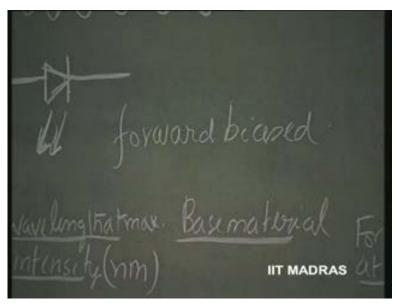
But, such a diode is, not a silicon diode. It is made out of, not group 4 element, which is silicon; 3 5 compound element, which is called, gallium arsenide or gallium arsenide phosphide or gallium nitrite, gallium phosphide. This material, when a P N junction is formed using this compound, 3 5 compound in the periodic table.
