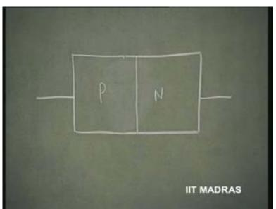
By formulating a PN junction like this, we are able to get the I V characteristics that is pretty close to the ideal diode; I V characteristic being the exponentially related characteristic between current and voltage. Now, apart from that, we would like to see what other terminal characteristics the diode represents. When it is a PN junction like this, at the junction, we have a region depleted of carriers, free carriers. This region is called depletion region.
