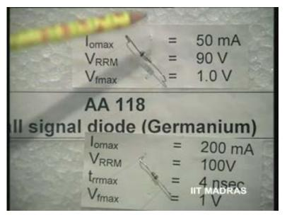
And the next one, the next one is a small signal silicon diode. Again, operating current, maximum forward bias current, maximum, is of the order of 200 milliamperes; peak inverse voltage rating is about 100 volts and is supposed to be a fast diode; and therefore, this recovery time from forward bias mode to the reverse bias, there is a delay time of the order of 4 nanoseconds.
