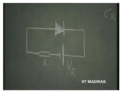
But therefore, the voltage across this is going to very near the voltage that I have applied; so, the magnitude of that voltage is going to determine the value of the capacitance. As the magnitude of the voltage increases, the capacitance decreases. This kind of nature, this capacitance, is of the order of picofarads. So, this diode therefore is called varicap or varactor diode; varicap - variable capacitance; so, either you call it varicap - variable capacitance or varactor diode.
