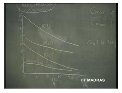
So, maximum to minimum, you should have normally as high ratio as 5; typical. It is a good varactor diode. And the maximum value of the capacitance itself depends
