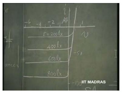
This, this value of current is going to be the short circuit current and this is the open circuit voltage for this photo diode or solar cell. And, the symbol for that is just the ordinary diode with light falling on the junction indicated by arrows; so light is falling on the junction as indicated. That is a photo diode symbol.
