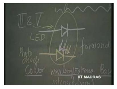
This light, magnitude, intensity, is dependent upon this current. And the current generated here depends upon the illuminance level of this here. So, in turn, you have a generated a current dependent upon this current and these two are perfectly isolated. So, this can be in one circuit and this can be in another circuit. This can be in, let us say, high voltage circuit this can be in the low voltage circuit, which is measurement circuit.
