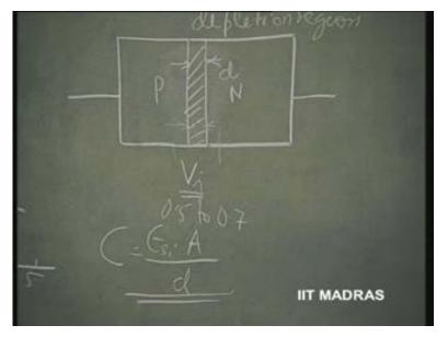
Parallel plate capacitance is nothing but the distance between the parallel plates which is d, coming in the denominator, epsilon, into Area of the capacitance plates. So, this constitutes the effective junction capacitance and this depletion layer width is dependent upon the reverse bias voltage that we apply; and therefore, if we apply a reverse bias voltage which is very large, depletion layer width increases, and therefore, the capacitance decreases.
