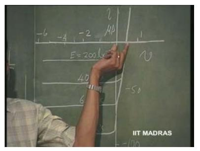
So, this is the open circuit voltage and therefore it can be used as a voltage source, a battery. That function of this diode, photo diode, is known as solar cell. That battery, which you can sustain by giving an external source of energy to the junction constantly, that junction voltage for silicon, is typically around point 5; and you can now find out that of your own.
