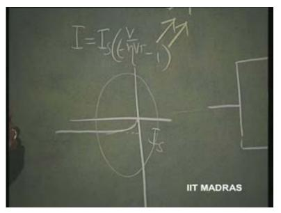
Now, what happens if I make light fall on this junction. So, that means, there should be a facility to expose the junction to light. So, that is the constructional feature of a photo diode where this junction is physically exposed to light; which means, these diodes will have a sort of glass window, which will expose the junction directly to light.
