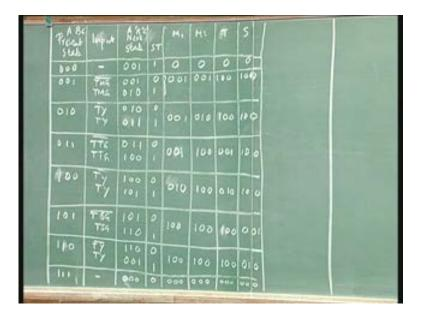
Finally 1 0 1, 1 1 0, TY bar, TY. 1 1 0, 0 0 1, goes back to the starting state 0 1, 1 0 0, 1 0 0, 1 0 0, 0, 0 1 0 and finally it is 1 1 1, it is not going to happen so irrespective of that reduce the don't care, we will put it 0 0 0 and all the signals will be 0. You make all zeros so that no problem occurs if it comes to this state. This it the state table or transition table if you want to call it or whatever.
