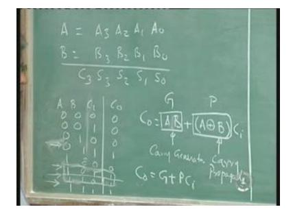
Let us use the 4-bit adders again A and B A is equal to  $A_3 A_2 A_1 A_0$  and B is equal to  $B_3 B_2 B_1 B_0$  these are the two bits you are going to add to get the sum  $S_0 S_1 S_2 S_3$  and  $C_3$  would be the fifth bit that we need. When you add two 4-bits you need a fifth bit and that fifth bit comes under this  $C_3$ .
